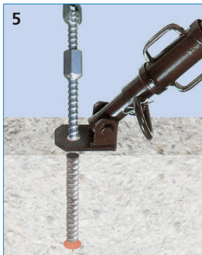
Screwing in the flexible screw-on-set.
